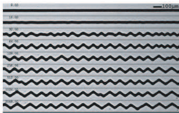
FIG. 1. Time evolution of a zigzag wall. The numbers located on the left side indicate times after applying the electric field.
